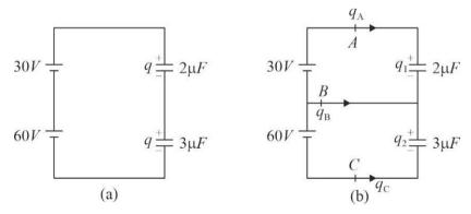
Refer Figure (a), when switch is open both capacitors are in series. Hence, their equivalent capacitance is
